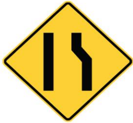
RIGHT LANE ENDS MERGE LEFT
